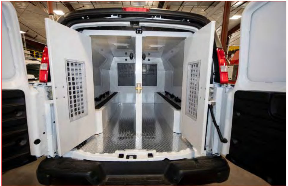
The new K9 Unit is divided into four compartments, with driver/passenger space, prisoner space, police dog space, and an equipment space in the back. Photo by Paul Arbogast.
