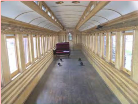
Interior of RGS coach 252, awaiting seats. The interior is finished as original, with ash wood, oak flooring and operating clerestory windows. Jim Pettengill photo.
