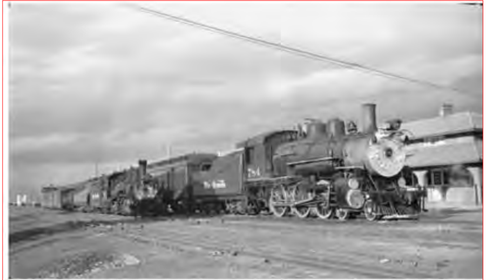
November 21, 1951. Denver and Rio Grande Western standard gauge locomotive 454 (2-8-2), with The Mountaineer passenger train, and narrow gauge locomotive 784 (4-6-0), with five freight cars, wait at the depot in Montrose (Montrose County), Colorado. Tanks are in the distance. Photo taken by Robert W. Richardson.
