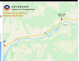
miles from Mile Point 75.4, east of Parachute, to MP 81.6, just east of Rulison. Work will include a 2" hot mix asphalt overlay, installing new guardrail, leveling asphalt at select locations, replacement of bridge rail and striping. Crews will repave the on and off-ramps at exit 81 (Rulison) as part of the project.
