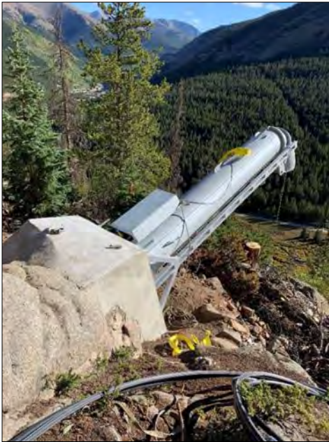
Gazex avalanche control unit used to mitigate snow slides on US 50 Monarch Pass, in Chaffee County. Courtesy photo.
